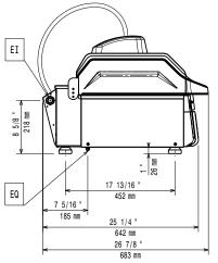
Electrical inlet (power) Electrical Outlet EO
